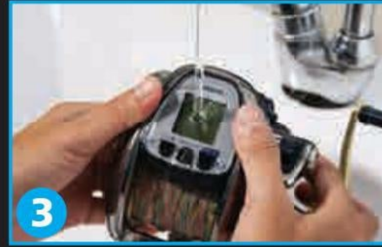
3 Quick run through of low pressure water on screen (not more than 3 seconds)
