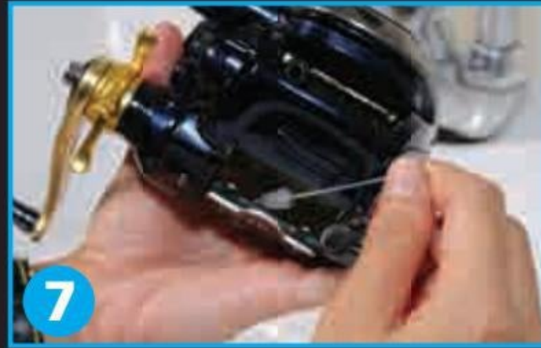
7 Use a tube brush to brush small accessible area (reel seat, line guide area) to ensure removal of remaining salt
