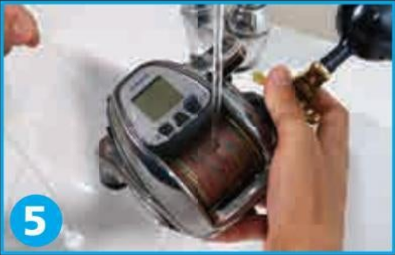
5 Engage clutch and pull out 2-3 meter of line while running low pressure water
