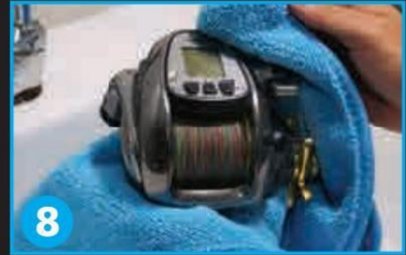
8 Use a wet cloth to wipe down the whole reel to ensure remaining salt and bait is removed
