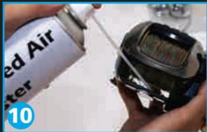
10 Use an air duster to spray difficult access areas to clear off water droplets
